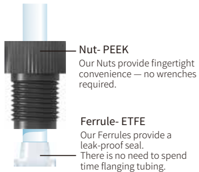
WD06B-5/16-24-K-black PEEK Flangeless Nut YK-048-F ETFE Ferrule For 4.8mm O tube
